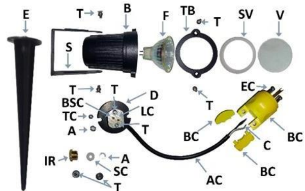
Fig. 5. Explosion diagram of the outdoor parts of the luminaire. Source: Own Elaboration
